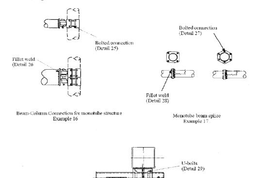
Beam-Column Connection for Truss Structure Example 18
